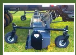
4 Wheels for Deck Height and Flotation
