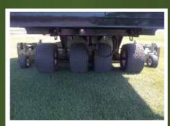
4 Turf Wheels for Flotation and Low PSI
